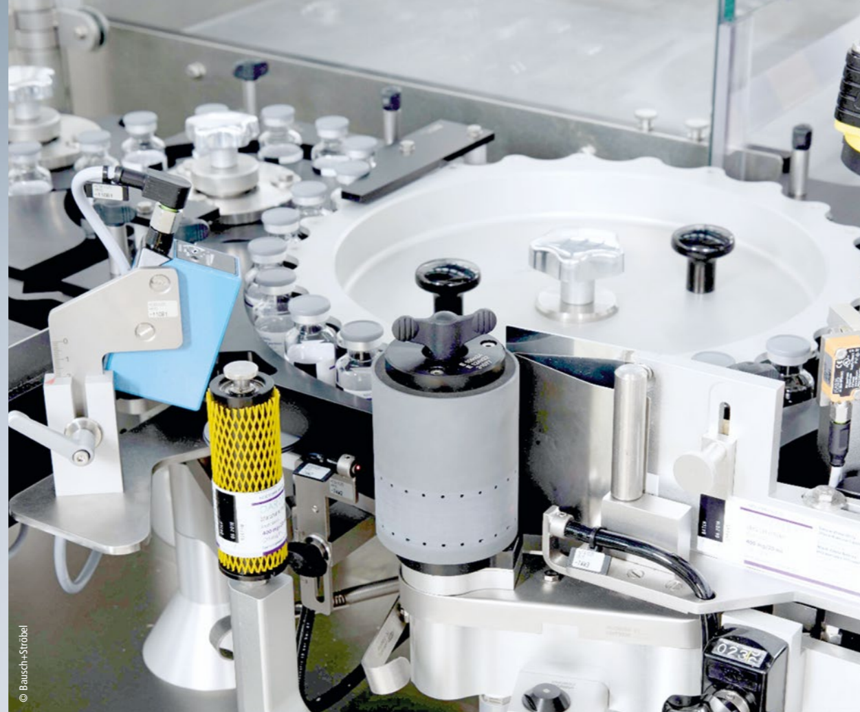
The way the vials are handled within the labeling machine is designed to ensure that neither the object nor the applied label is damaged, based on advanced features including the high-performance motion control.
