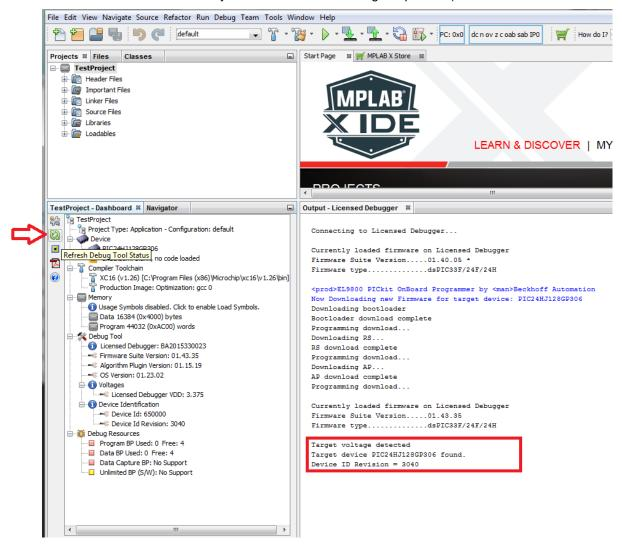
This confirms a correct communication between MPLAB X IDE and the Evaluation Kit.
