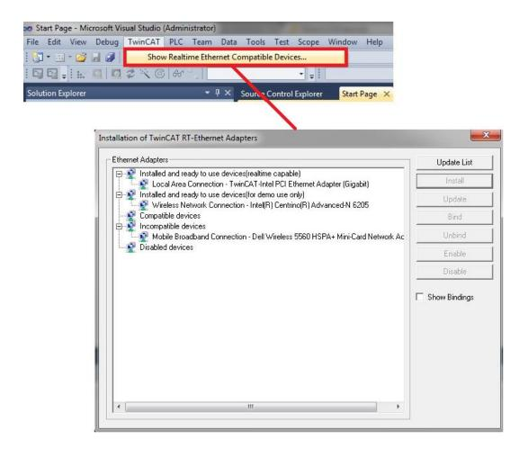
Select the network card that will be used as EtherCAT Master for testing purposes, and click on "Install".
