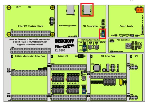
Power the Evaluation Kit on with a standard 24V power supply.
