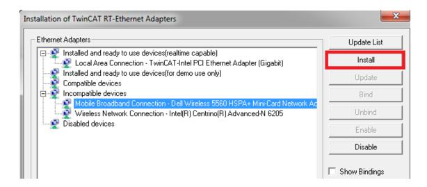
**NOTE**: If a network card is listed under "Incompatible devices", this does not mean that the card cannot be used as EtherCAT Master for testing purposes. It only means that this card will provide only weak real-time capabilities. For testing purposes this is more than enough, therefore you can proceed with the installation.
