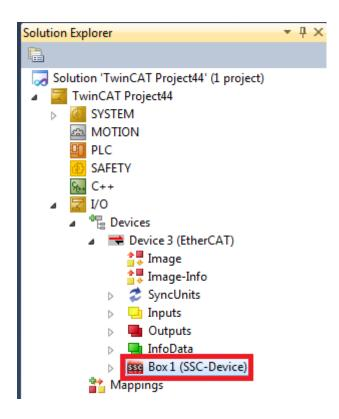
**NOTE**: The particular icon and name of the detected device are not relevant, as they depend on the previous status of the Evaluation Kit. The important thing is that a slave "Box m (xxxx)" is detected.
