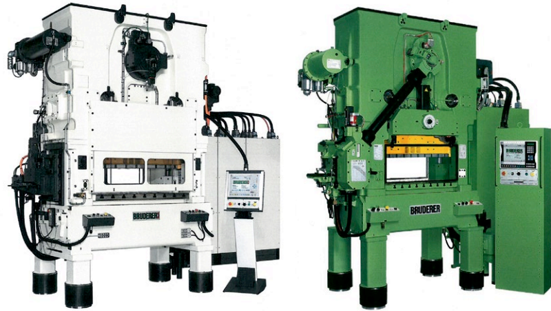
A recent stamping machine in the BSTA series (BSTA 810, left) and the first BSTA 500 stamping machine supplied with a Beckhoff control system in 1999 (right)
