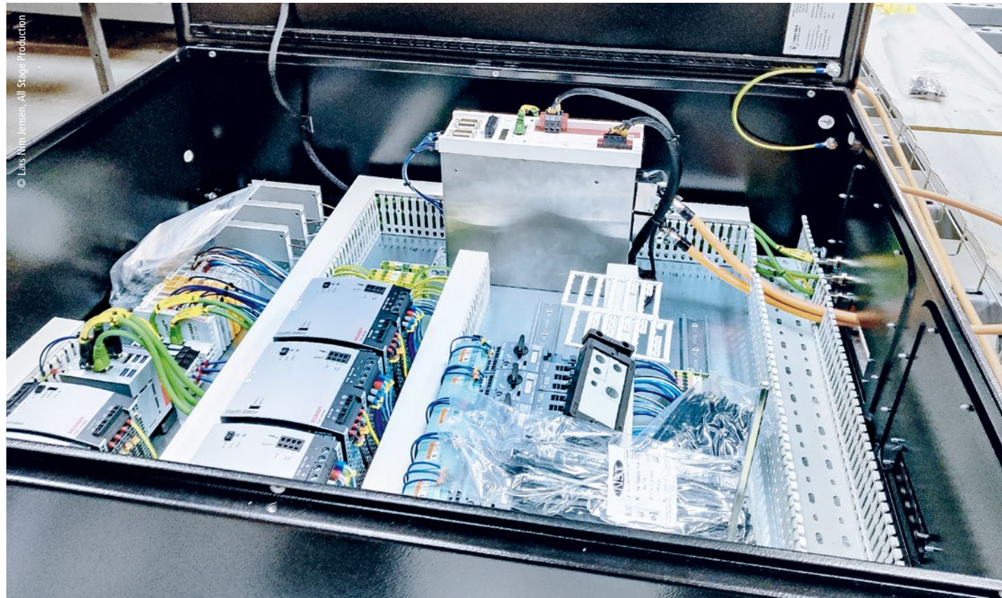
Control cabinet during assembly with a two-channel AX52xx servo drive, a C6017 ultra-compact Industrial PC, and several PS3000 power supply units for the AMI8100 distributed servo drives
