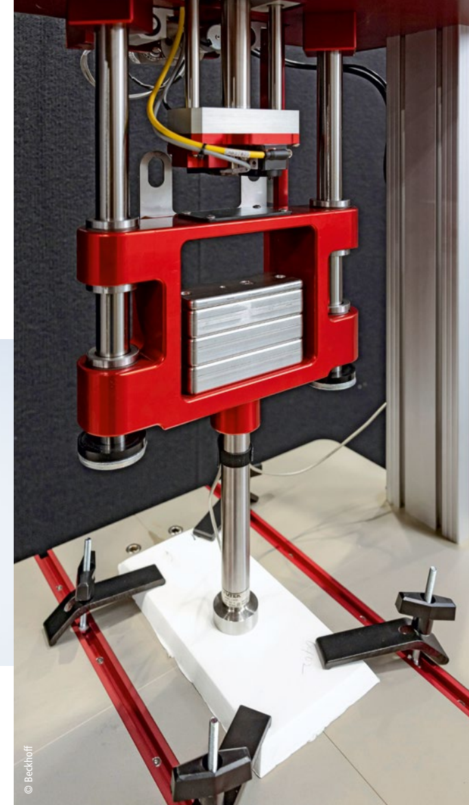
EtherCAT communication ensures synchronization of load versus position for test integrity.
