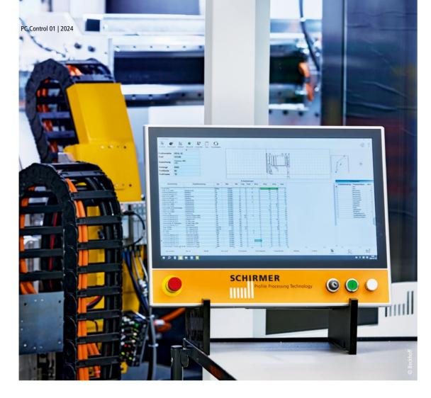
The complete machine is set up and operated via a customerspecific Beckhoff Control Panel
