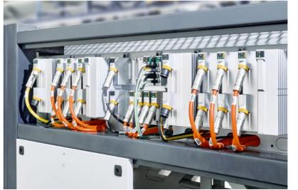
Double-row baseplate of the MX-System: The open installation on the base frames simplifies machine wiring and facilitates diagnostics. worldwide | germany PC Control 01 | 2024 worldwide | germany
