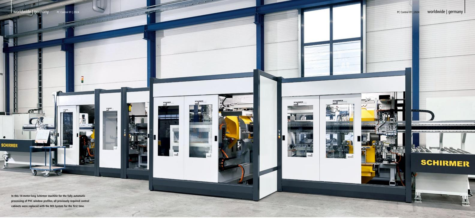
MX-System for a window profile processing machine
