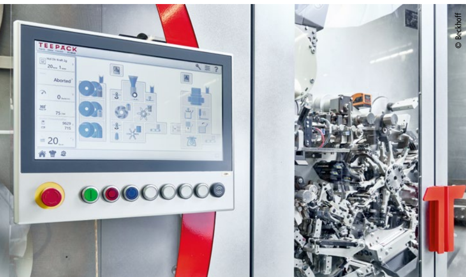
The CP39xx multi-touch Control Panel with push button extension enables optimum operation and monitoring of machine processes.
