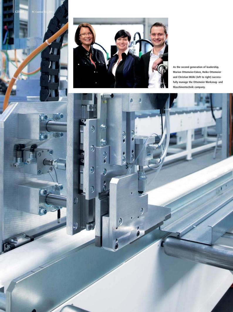
A door frame consists of two side jambs and a header. All three elements are made from beveled sheet metal and are mitered. The steel frame processing line for Hörmann consists of four saws, two gantries for material loading and several roller tracks for material handling. In addition to the saw unit the line also includes a laser cell with a special material supply concept and was extended with a complex punching machine during the course of the project.
