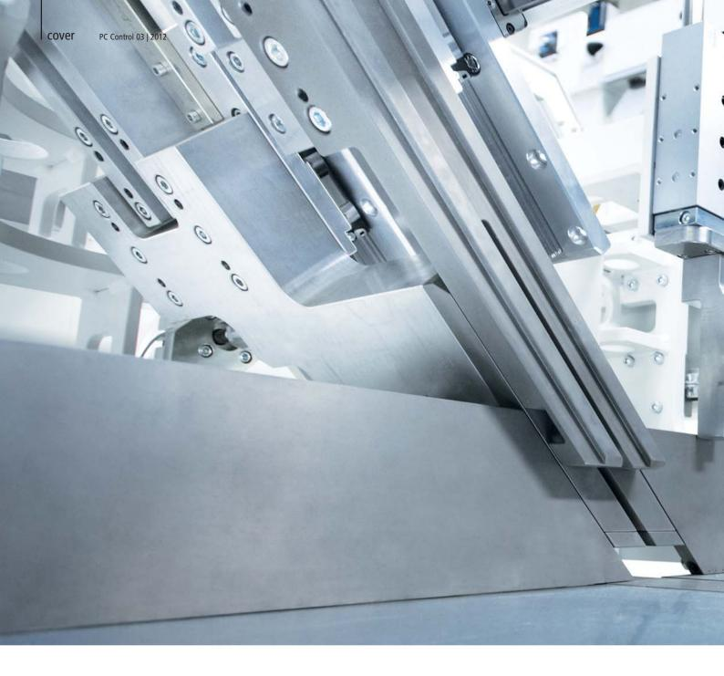
Steel frame processing line: PC-based Control replaces conventional clamping technology with high performance servomotors
