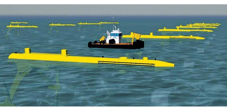
Model of a tidal turbine "farm" for energy generation in the North Sea. The SR2000, which is currently being developed by Scotrenewables, is expected to have a rated capacity of 2 MW at a flow rate of 3 m/s.
