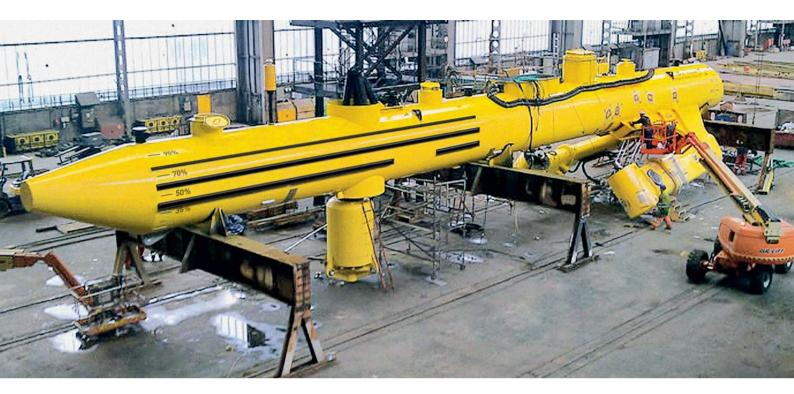
Construction of the tidal turbine, which was specially developed for the demanding conditions in the North Sea.
