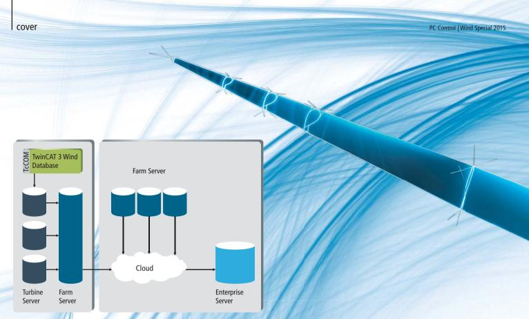
Fig. 5: The system data can be consolidated on central servers for higher-level analyses.
