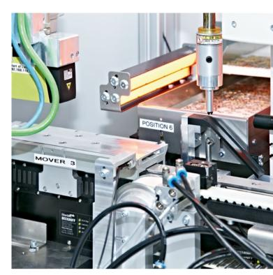
The decoupling of transfer system and process stations is particularly important in the assembly of small parts.
