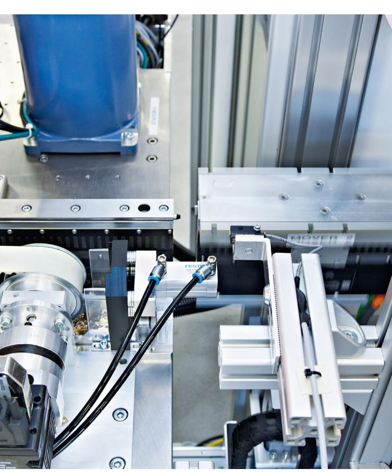
Credimex uses the extremely flexible XTS as a linear transfer system with mover return via a spindle-driven system located underneath.
