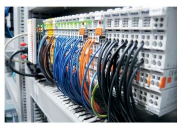
The modularity of the Beckhoff terminal system allows subsequent changes and additions at any time and little cost.
