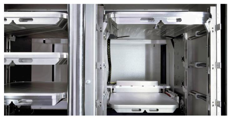
Optional MetalFAB1 storage module for storing workpieces
