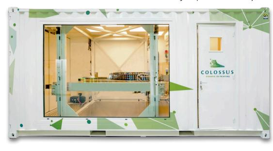
"Transparent production" in a container allows a free view of the 3D printer from IMA and is intended to give the public a clear idea of the way it works.
