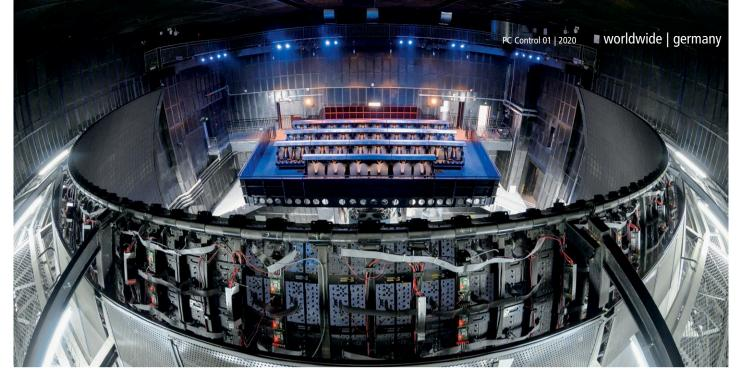
The Hexaflite® Flying Theater consists of a platform that is movable with six degrees of freedom and surrounded by a circular screen, resulting in a viewing angle that's 180 degrees horizontally and 110 degrees vertically.
