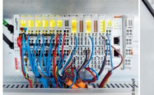
To calculate the exact positions in real time, the researchers rely on XFC's timestamp technology and the relevant EtherCAT Terminals.
