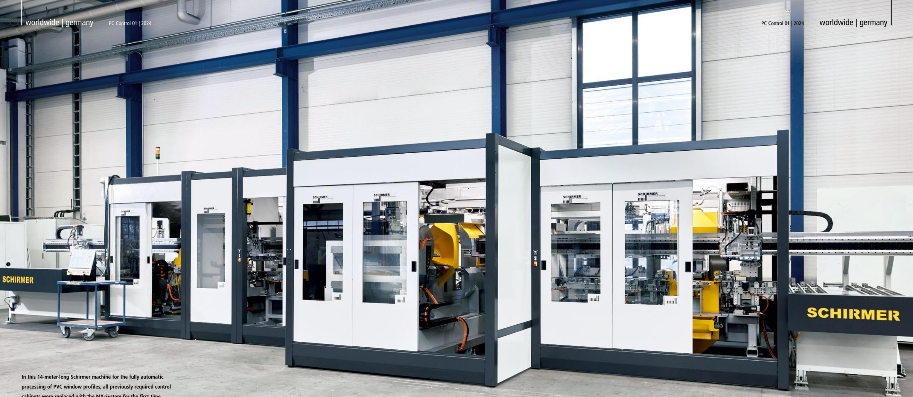
In this 14-meter-long Schirmer machine for the fully automatic processing of PVC window profiles, all previously required control cabinets were replaced with the MX-System for the first time.
