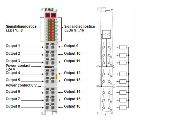
EL2869 | HD EtherCAT Terminal, 16 digital output channels, 24 VDC, 0.5 A, with channel diagnostics
