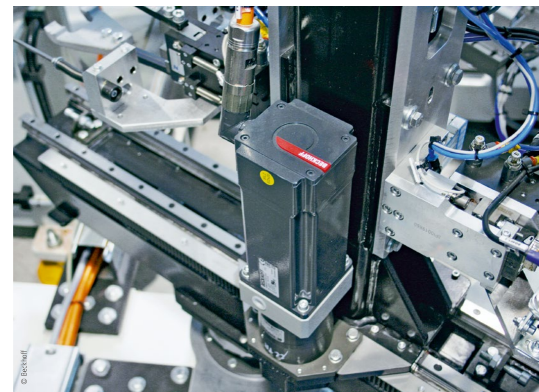
The distributed connection concept based on EtherCAT P and the compact AMP8000 servo drives save valuable space in the machine.
