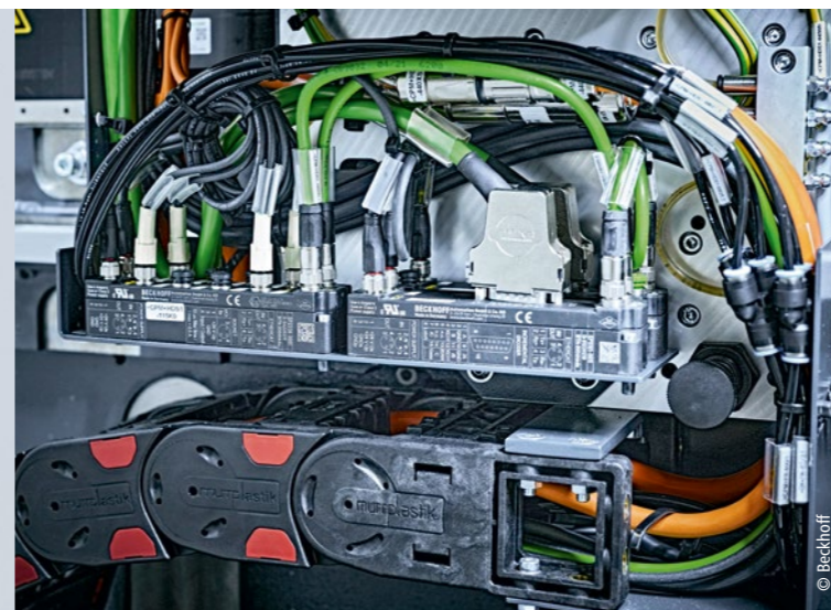
The wide I/O spectrum of IP20 EtherCAT Terminals and IP67 EtherCAT Box modules (here: EP2338 and EP5101 in the BLS 500) facilitates the modularization of Manz systems.
