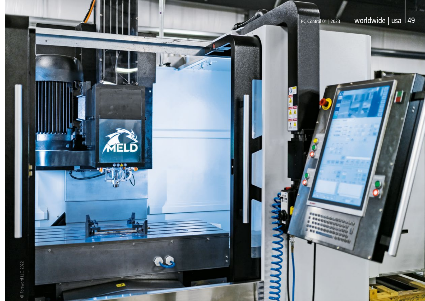
A B8 machine from MELD prepped and ready to print
