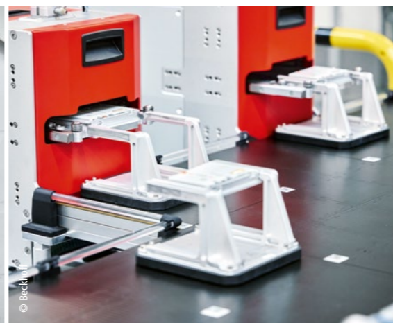
AA3000 electric cylinders are used to insert the terminal carrier; AA1000 linear actuators are used to lower the contact pins.
