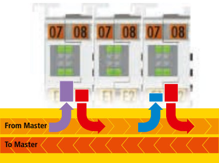
FMMU (fieldbus memory management unit): Telegram processing completely in hardware
