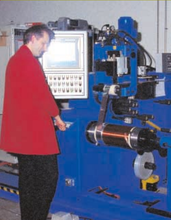
Christoph Müller, manager of electrics and software at Tuboly, operates a transformer winding machine. Operation is largely automated.
