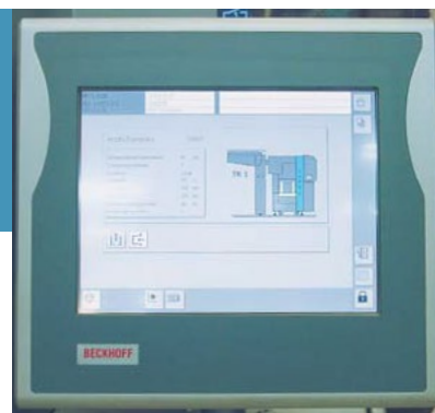
The Beckhoff CP77xx and CP69xx Control Panels are used as operating terminals and were manufactured as custom versions especially for Ferag. The CP62xx Panel PC version is also used.
