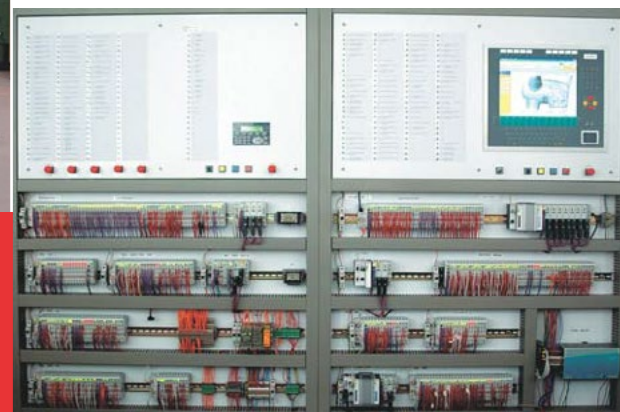
The M5000 test stand is used primarily for reducing the time for function tests and commissioning and for optimizing the operating procedures and control processes.
