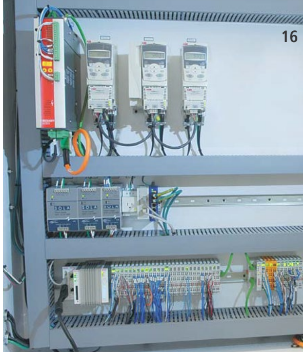
The redesigned Talon popcorn bagging machines are controlled by a CX1020 Embedded PC with TwinCAT NC PTP.
