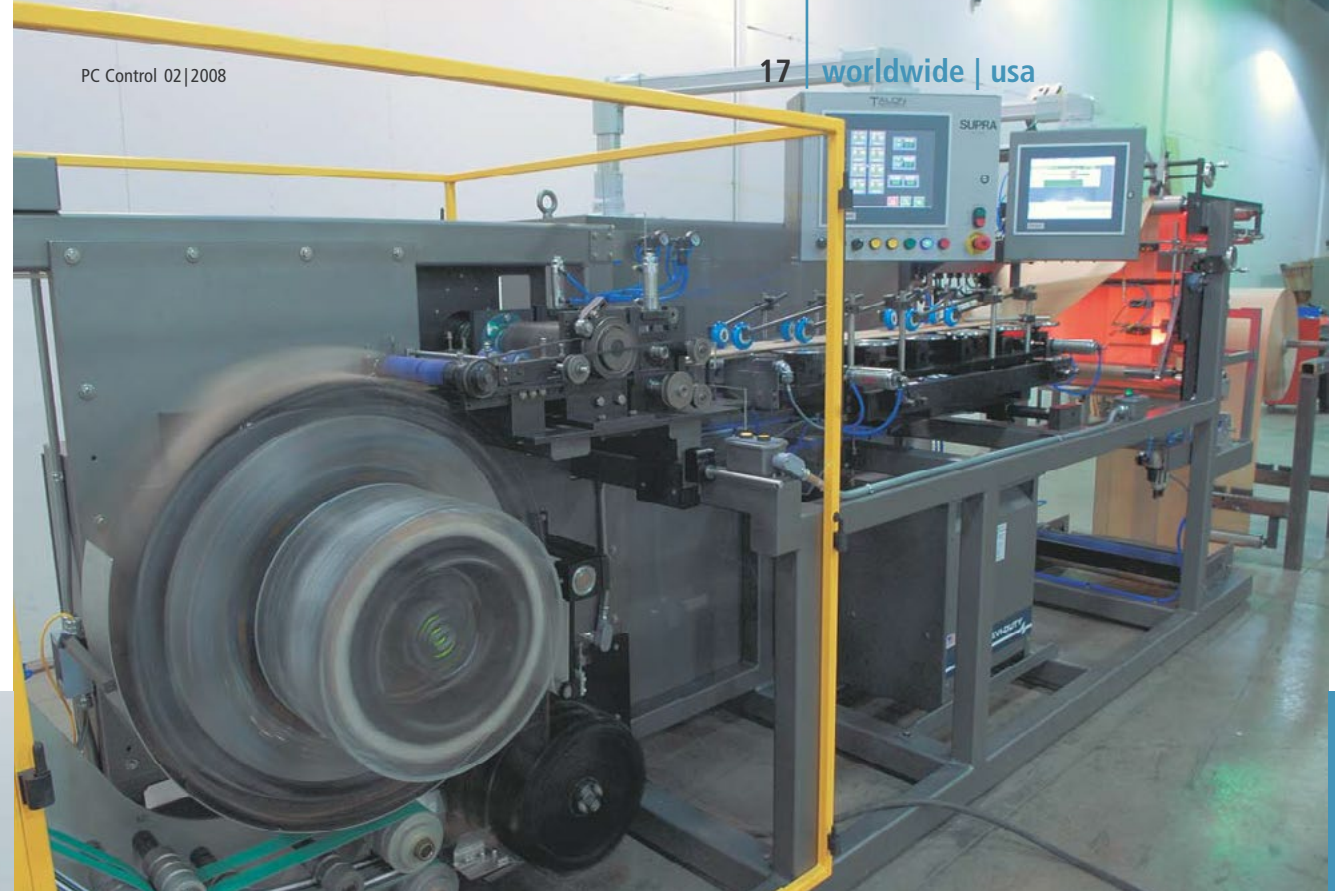
The PC-based control system offers maximum precision: The popcorn bags now have more precise cuts and a more consistent length.
