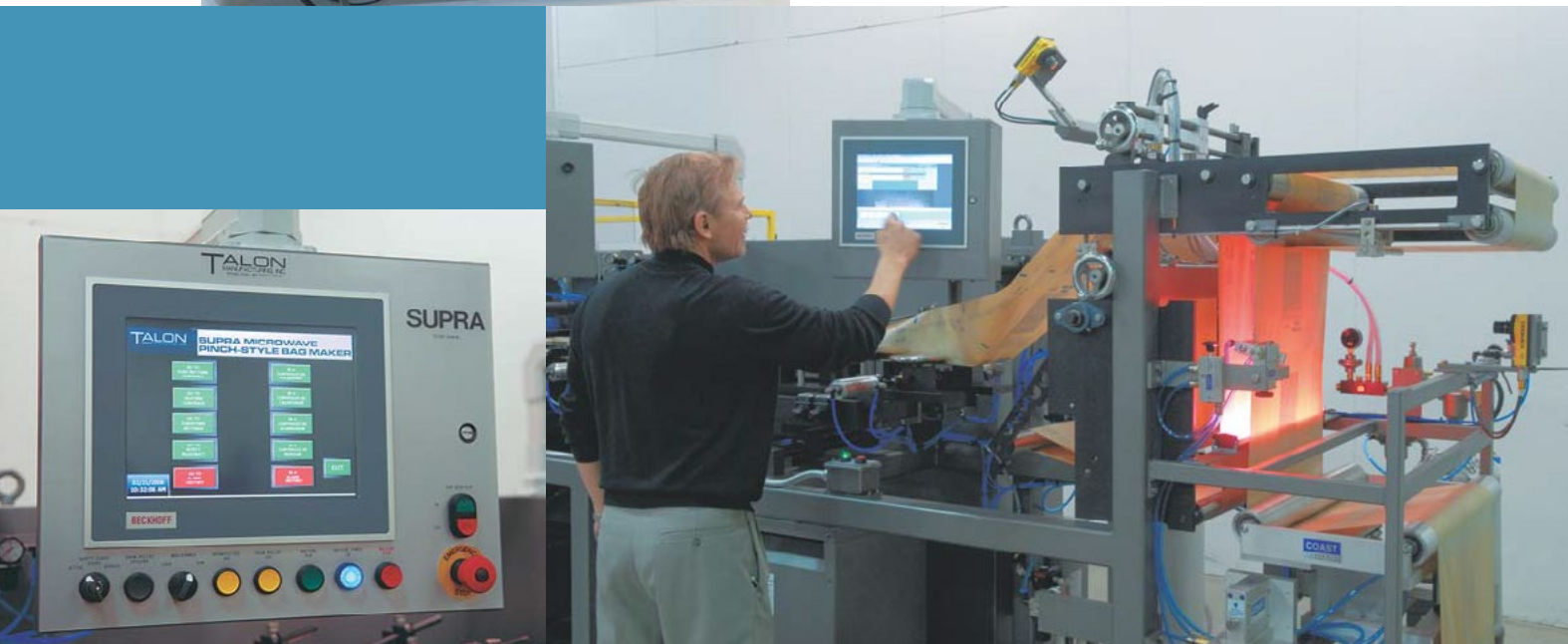
Talon uses CP62xx Panel PCs for "all-in-one" control and display devices and CP69xx Control Panels for simple display and control functions.
