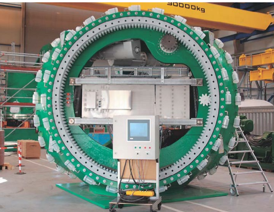
The M5000 test stand is used primarily for reducing the time for function tests and commissioning and for optimizing the operating procedures and control processes.
