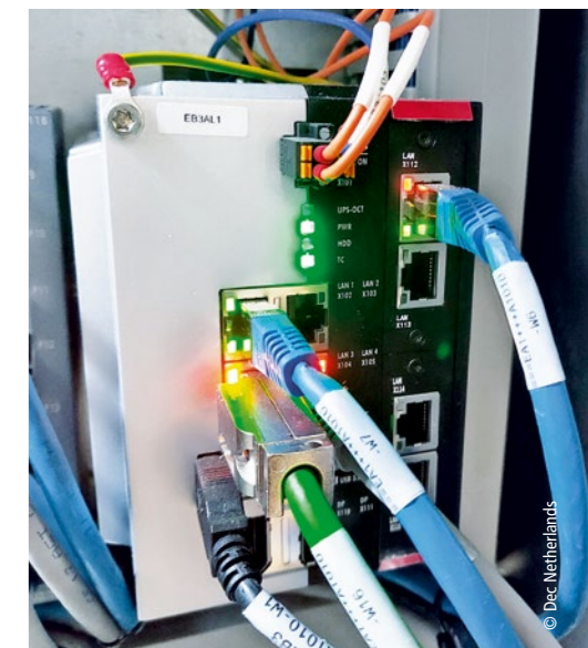
The C6032 ultra-compact Industrial PC with TwinCAT XTS Extension, Collision Avoidance, and NC PTP controls the movers precisely and without sloshing any liquids during start-up and braking.
