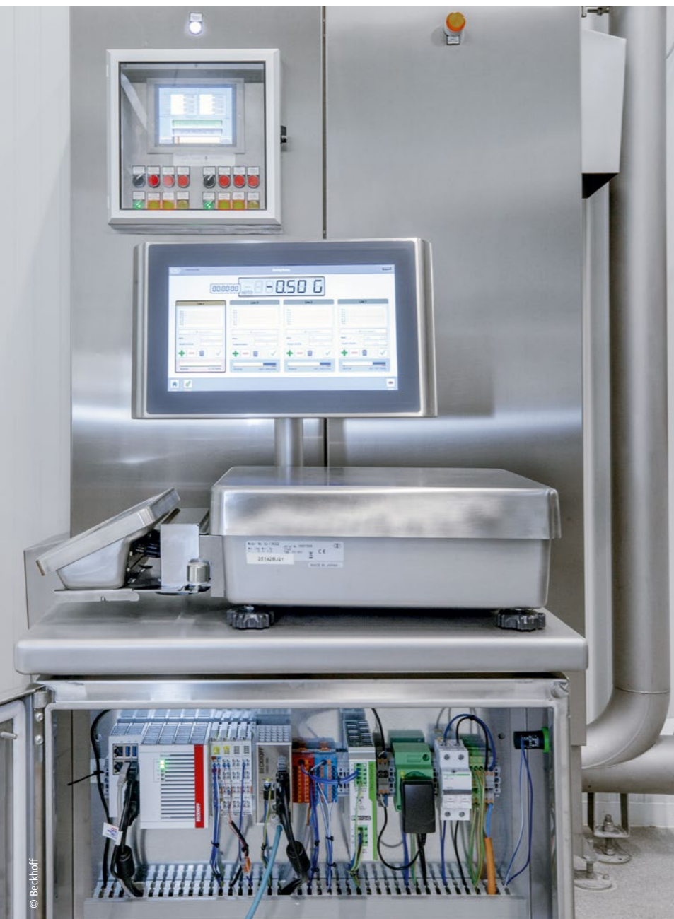
The previously manually adjusted dough dosing was converted to servomotor-based control including evaluation of all data in a cloud platform.
