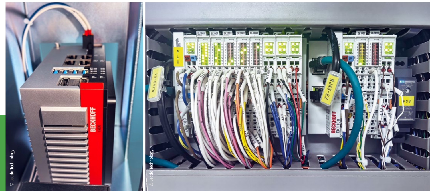
A C6030 ultra-compact Industrial PC with exceptional computing power and versatile interfaces is used as a machine controller for the dicing saws.
