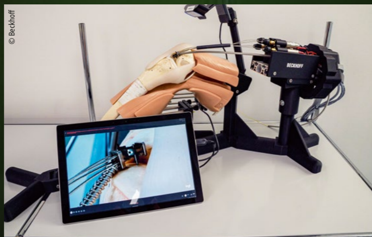
To perform operations correctly, flexible spiral spindles enable the miniature robot to be moved precisely inside the body.
