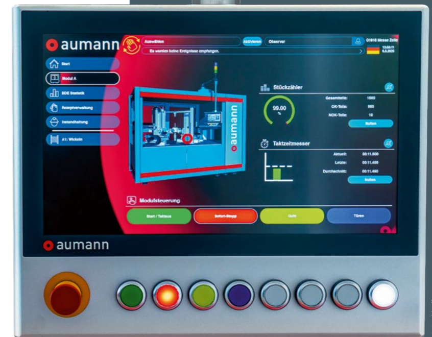
As the HMI for the new needle winding machine, the CP3916 multi-touch Control Panel was customized specifically for Aumann and tailored precisely to the application.
