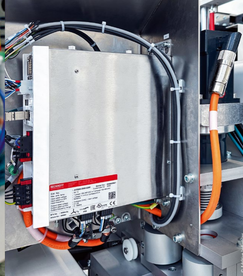
3D printing requires precise motion sequences, which Additive Industries realizes with AX5000 servo drives and AM8000 servomotors.
