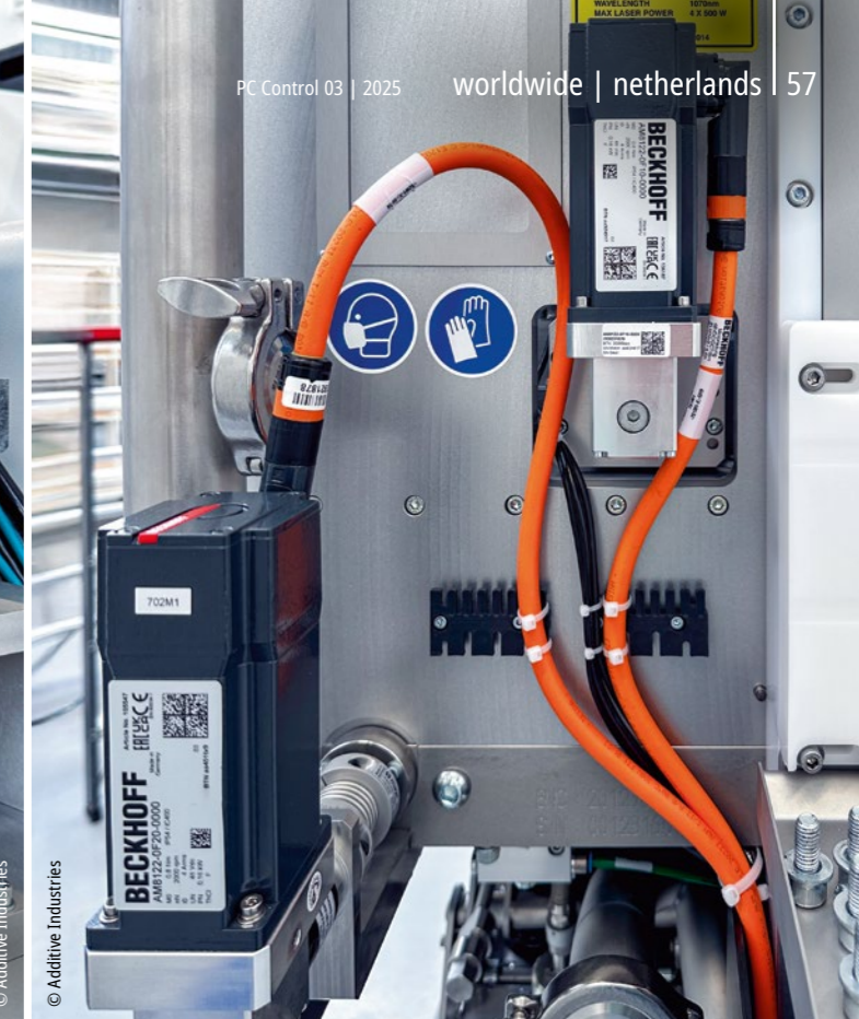
The axes of a 3D printer – which can number up to fourteen – are driven precisely and dynamically by AM8000 servomotors.
