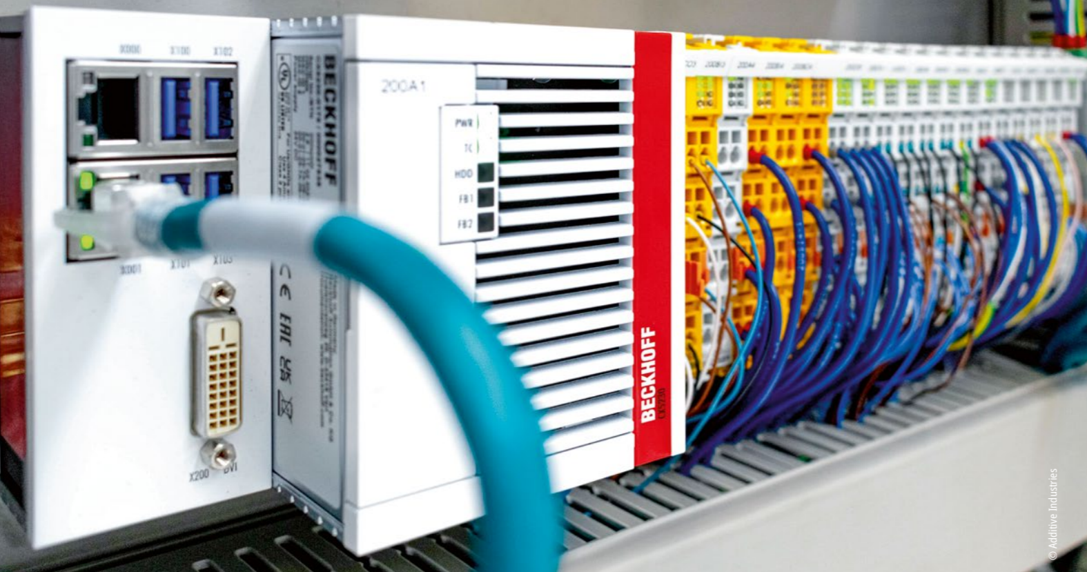
Additive Industries and Cordis rely on a CX5230 Embedded PC with TwinCAT for the control technology.
