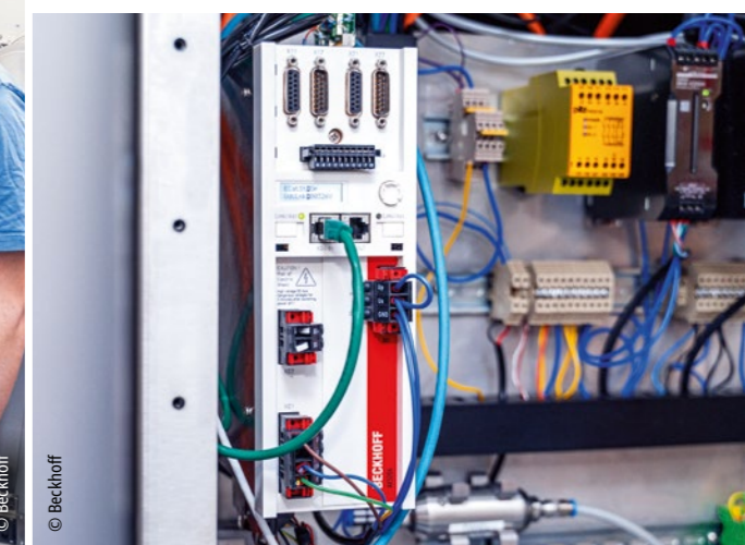
The 2-channel AX5206 servo drive ensures precise and dynamic movements.
