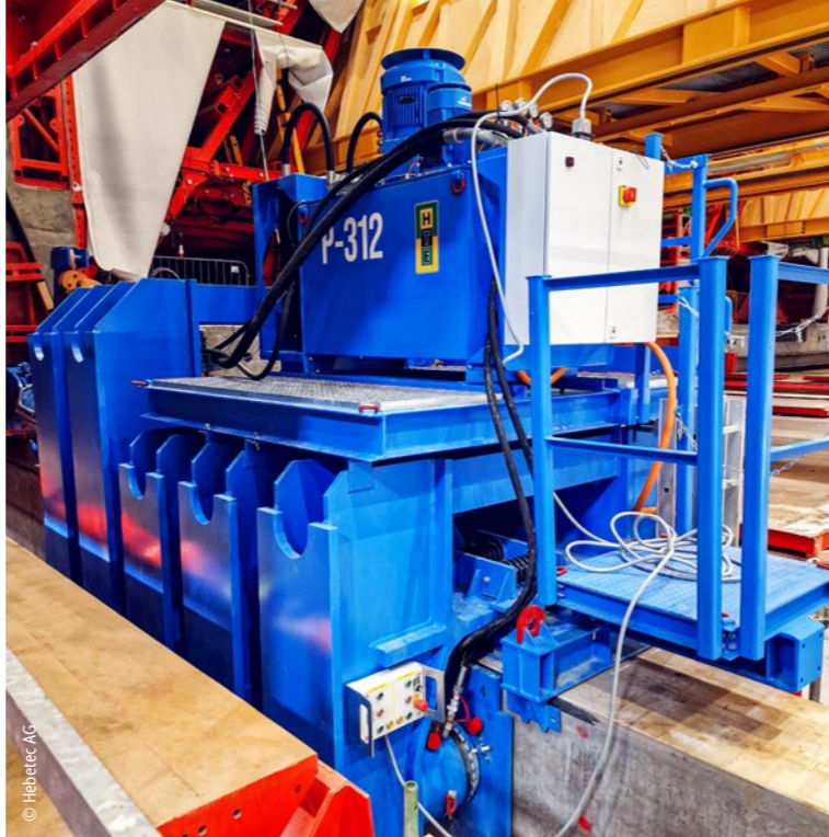
Six of these pushers, each with two cylinders, push the tunnel segments evenly over several hundred meters through a narrow gate into the dry dock during continuous production.
