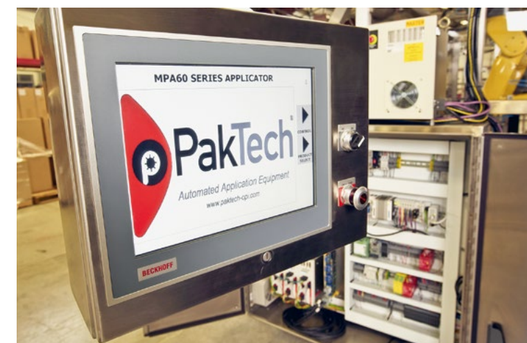
The MPA60 features the rugged CP6201 Control Panel for HMI hardware that's well-suited for demanding plant environments.
