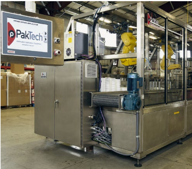
PakTech handle applicator for applying multi-pack handles on various bottles and packages
