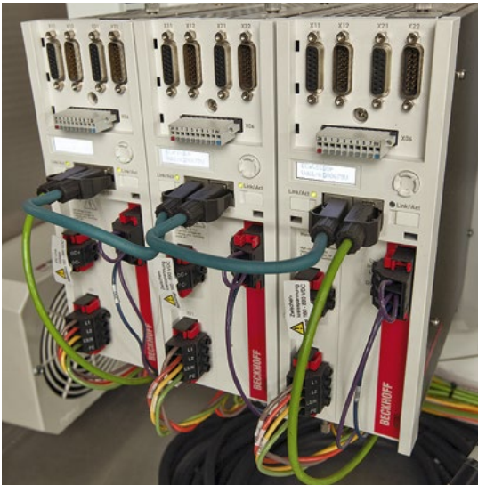
Paktech uses the two-channel, space-saving AX5000 EtherCAT drive.
