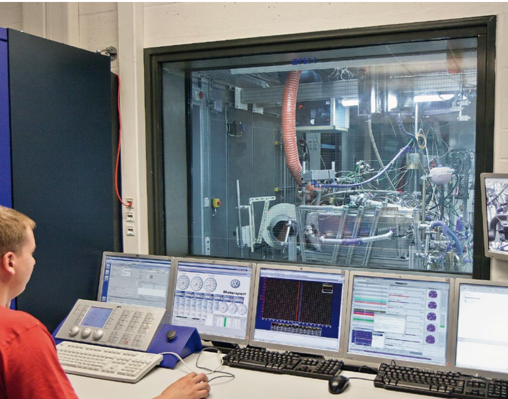
The engine experts from Volkswagen used TwinCAT HMI CE visualization software from Beckhoff to keep an eye on the processes.
