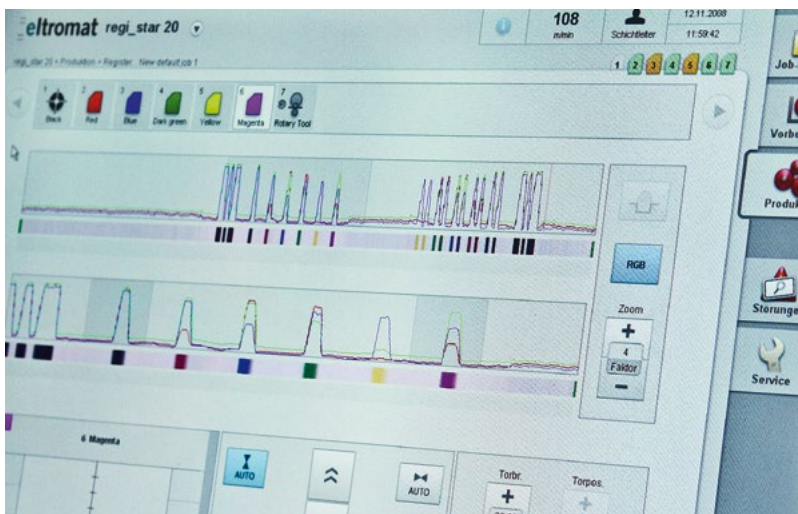
The print marks are detected quickly and precisely thanks to XFC technology from Beckhoff.
