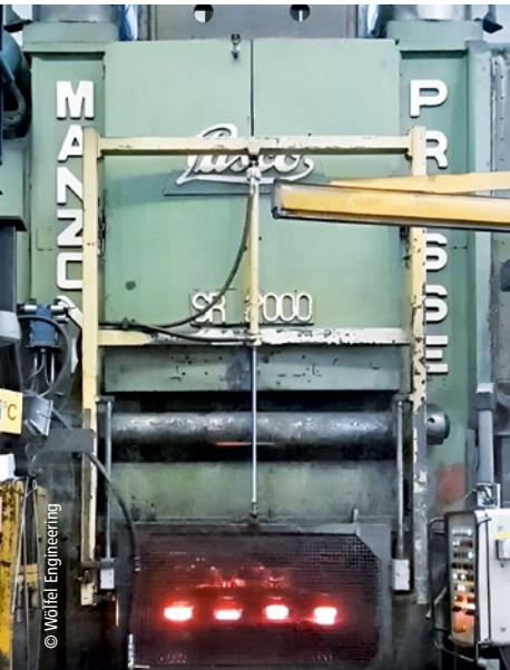
The eccentric press, which was installed in 1989 and weighs approx. 150 metric tons, has been modernized several times. In this context, the press was retrofitted with a customized condition monitoring system.
