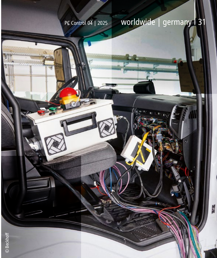
A compact control box is connected to the vehicle electronics via a vehicle-specific adapter cable set. The control box receives CAN messages modified with TwinCAT and feeds them into the vehicle communication system.
