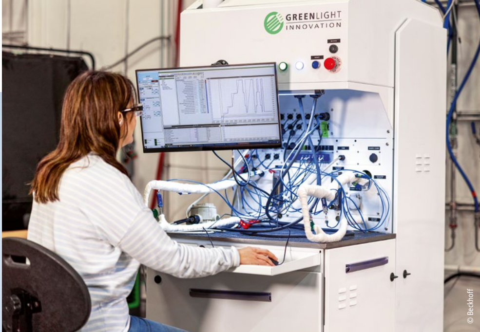
The Greenlight electrolyzer test station evaluates and validates performance, durability, and efficiency.
