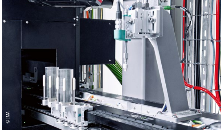
The assembled battery cells entering a test station
