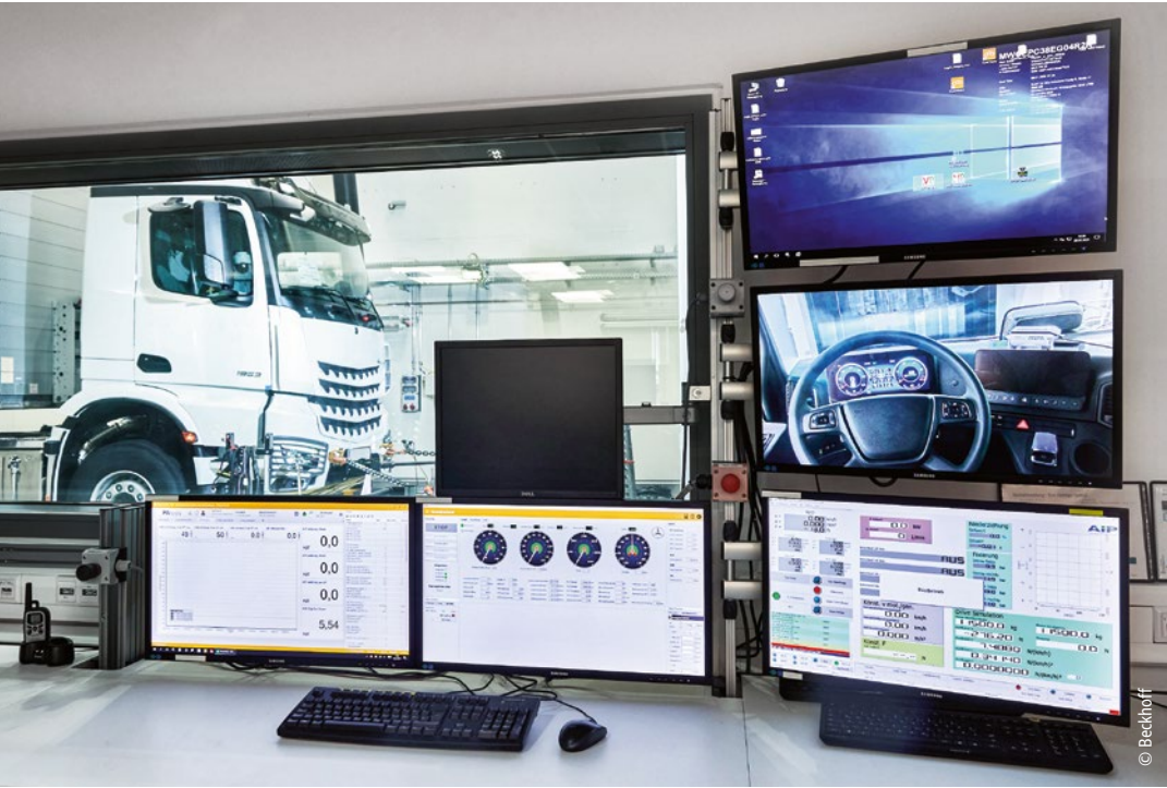
The fully automated test sequences are started and monitored via the control station; a camera installed in the driver's cab serves as a visual control point.
