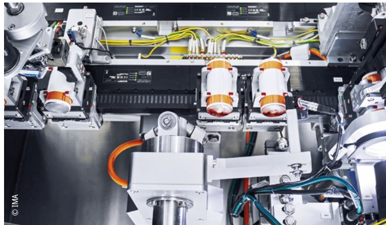
Transporting the battery cells attached to the XTS movers from one assembly station to the next
