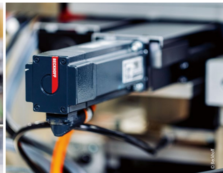
ELM7212 servomotor terminals and connected AM8100 servomotors control printhead positioning to ensure smooth overlay of multiple ink colors.
