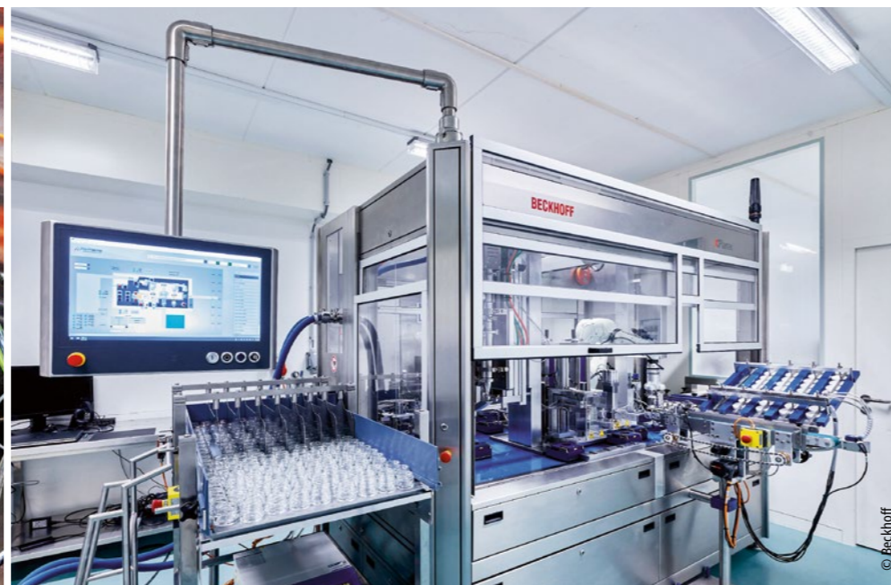
XPlanar increases the flexibility of the filling and capping line from Glanzer cosmetic engineering and Pro Pharma Automation to a high degree.
