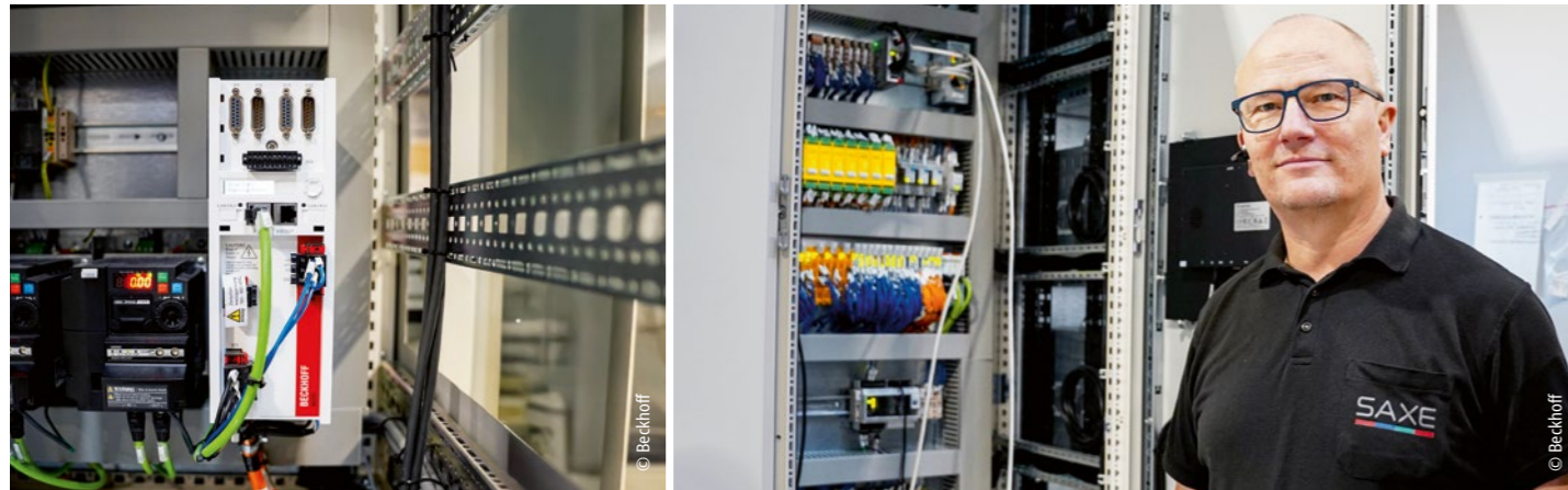
AX5203 2-channel servo drives in combination with AM8022 servomotors assure dynamic and synchronized movement for the take-out system.
