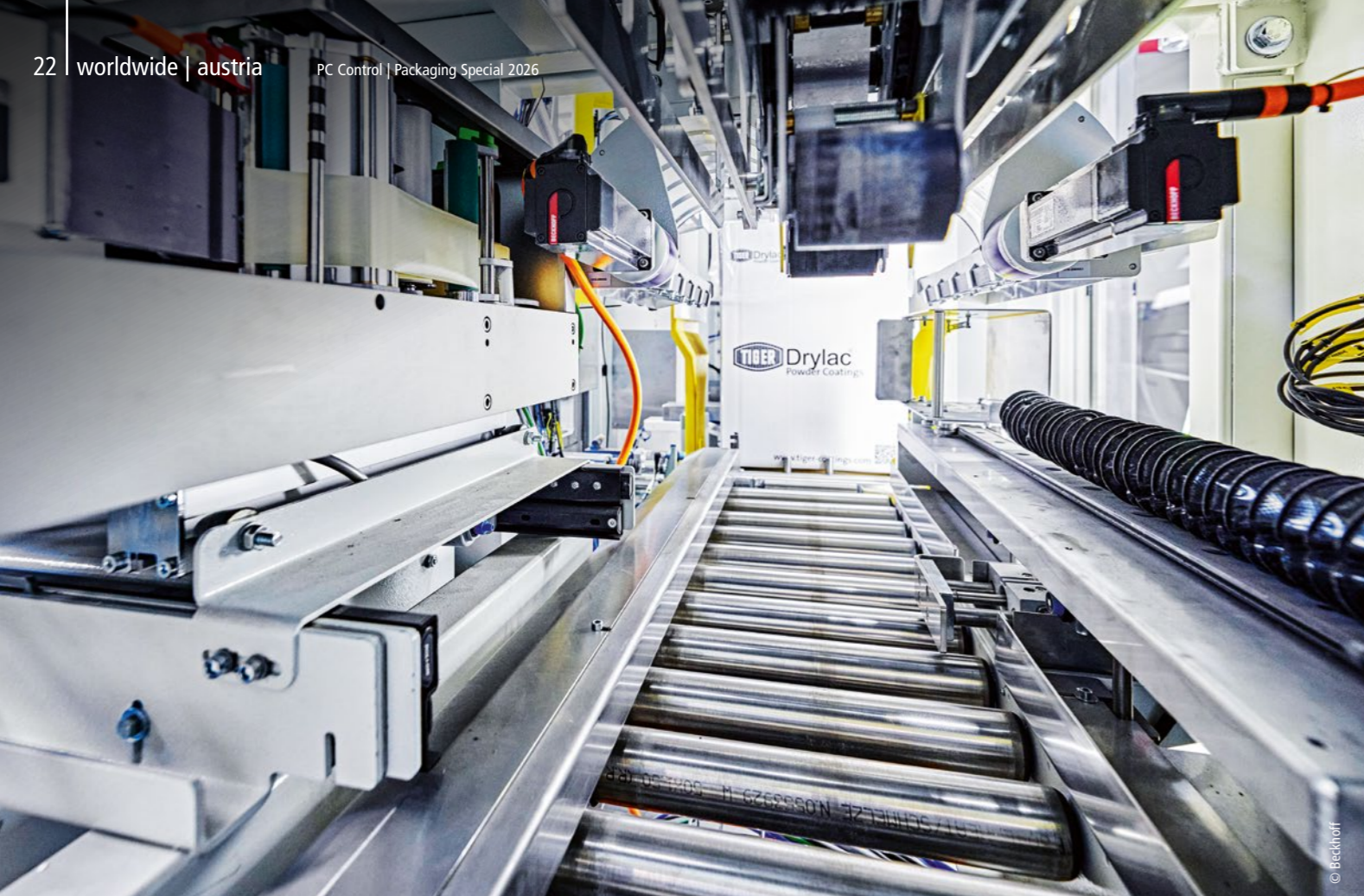
The system carries out various process steps fully automatically – from closing the inner bag and sealing the box to weighing, labeling, and palletizing.
