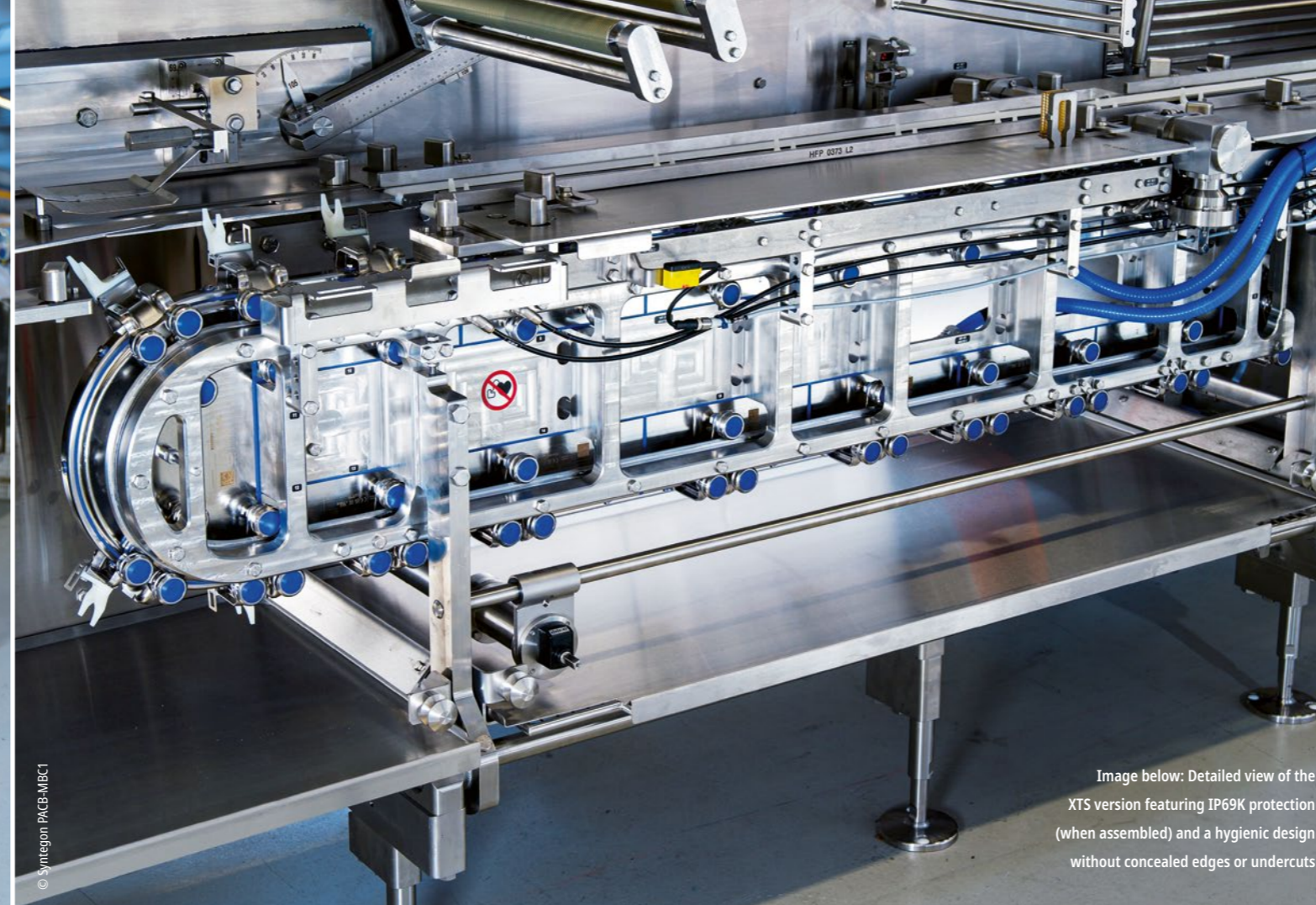
The XTS Hygienic linear transport system is key for the handling capabilities of Syntegon's horizontal flow wrapping machine in washdown design.
