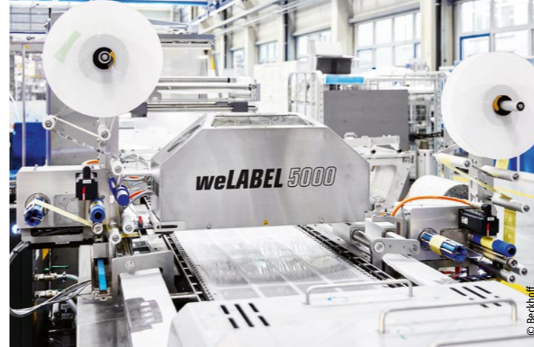
The packaging machines can be flexibly equipped with up to four weLABEL labelers (one top and one bottom web carrier in this case) as required.
